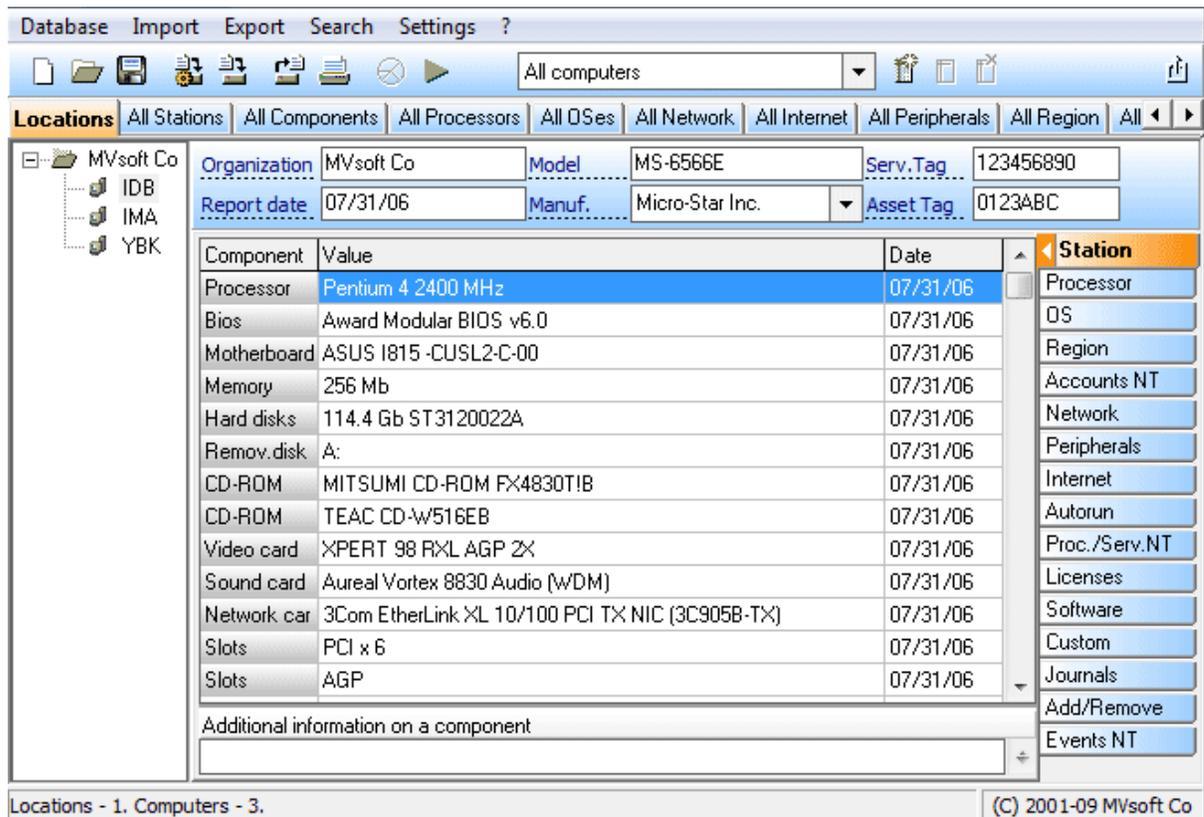
Left part shows enterprise structure as a tree of locations (subdivisions) and their computers, right one contains information about components, peripherals and software of selected computer. Both parts have context menus to perform the operations.
