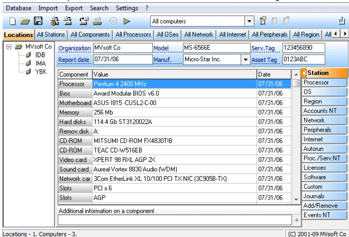
Table you will see represents data about computer station components. It is divided in 3 columns: [Component](#), [Value](#) and installation [Date](#). All operations with the data in that table are performed with use of a context menu available by right mouse button clicking.
